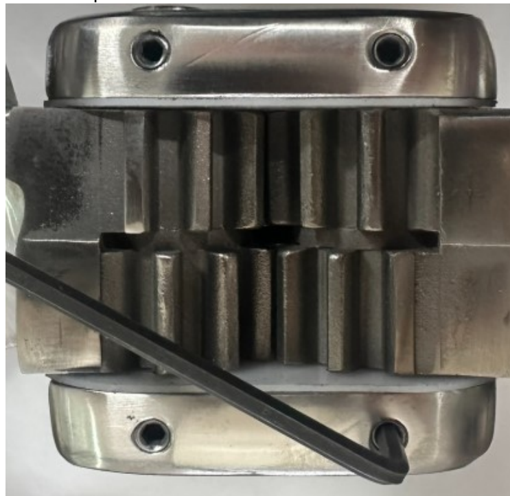
Removing the grub screws
