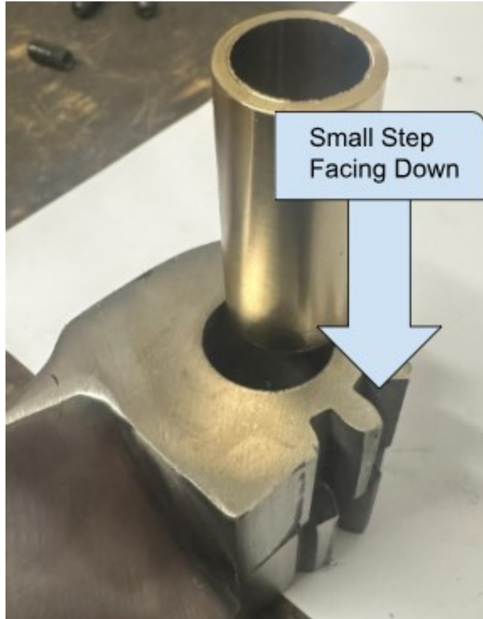
Replacing the Blade Bearing
