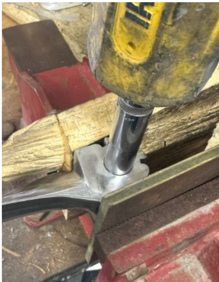
Removing the Blade Bearing
